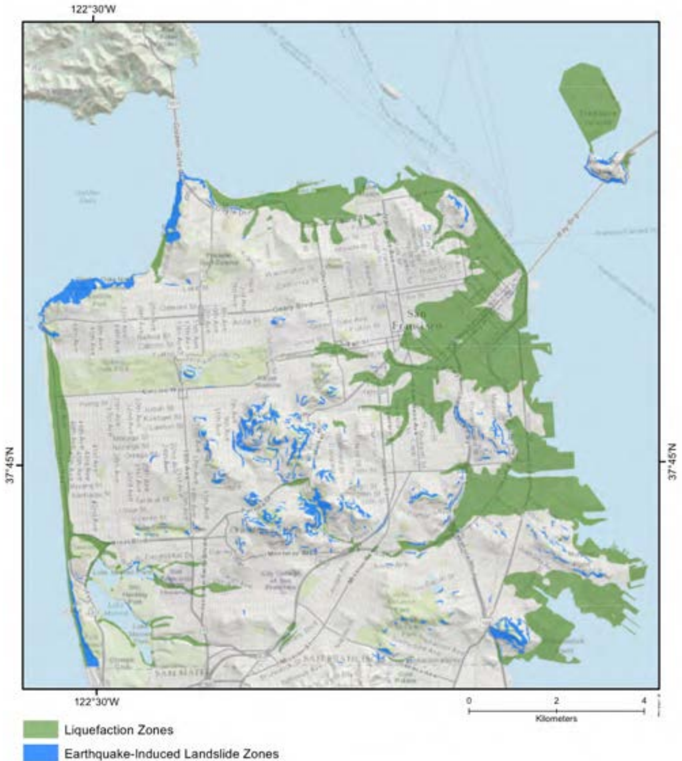
Figure 51. California Geological Survey’s Seismic Hazard zones map showing zones of required investigation for liquefaction and earthquake-induced landslides (map data from http://maps.conservation.ca.gov/cgs/information/warehouse/index.html?map=regulatorymaps ).
