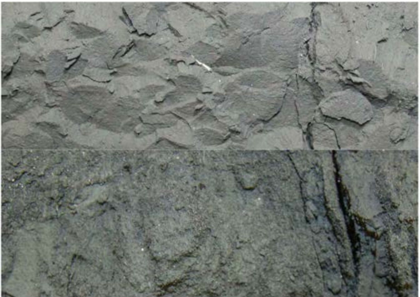
Figure 90. Top: Typical Young Bay Mud clay (15 m, 50 ft), Bottom: Typical estuarine clayey sand (29 m, 95 ft) (ENGEO, 2015).
