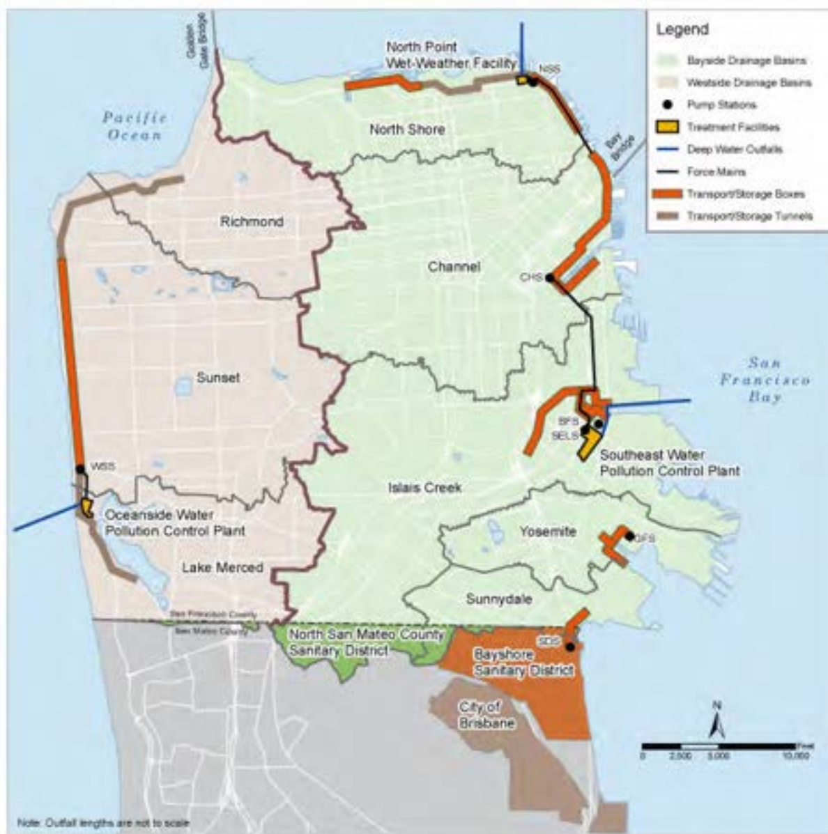
Figure 95. San Francisco Sewer System Drainage Basins and Major Sewer System Infrastructure. (SFPUC, 2018c).
