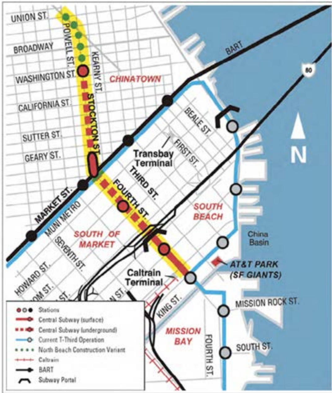
Figure 23. Central Subway railway alignment and new stations (San Francisco Municipal Transportation Agency, 2018).
