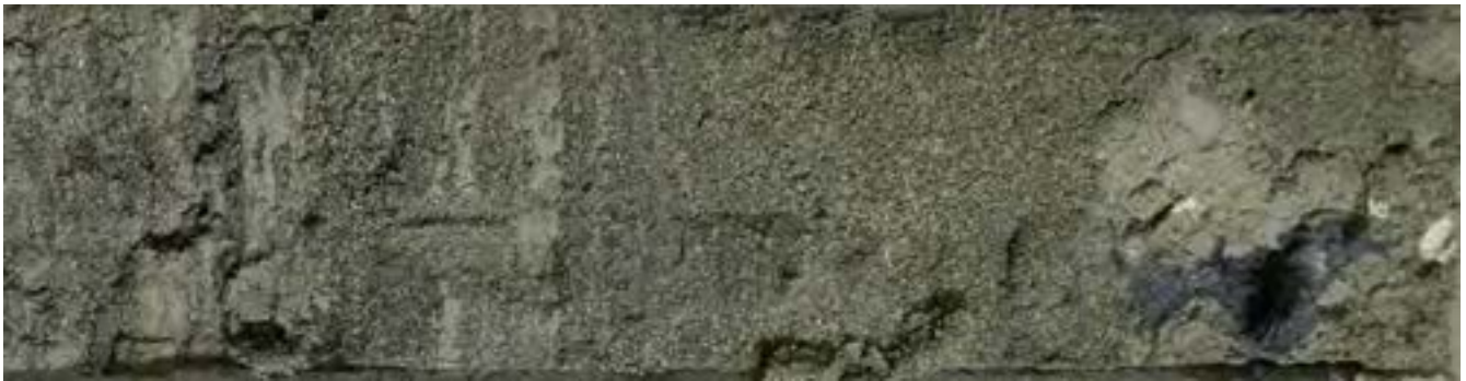
Figure 86. Fill sample from 9.1 to 9.4 m (30 to 31 ft) showing poorly graded sand with sharply defined clay and silt laminations (ENGE0, 2015).
